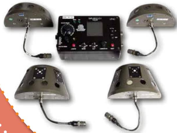
**STRUCTURE :** • 4 heads with laser and radar sensors, integrated on both left and right sides of the armored vehicle • 2 heads are installed on the front of the vehicle and 2 on its back side • Processing Display and Command Unit – UPAC • Connection cables for the sensor blocks.
